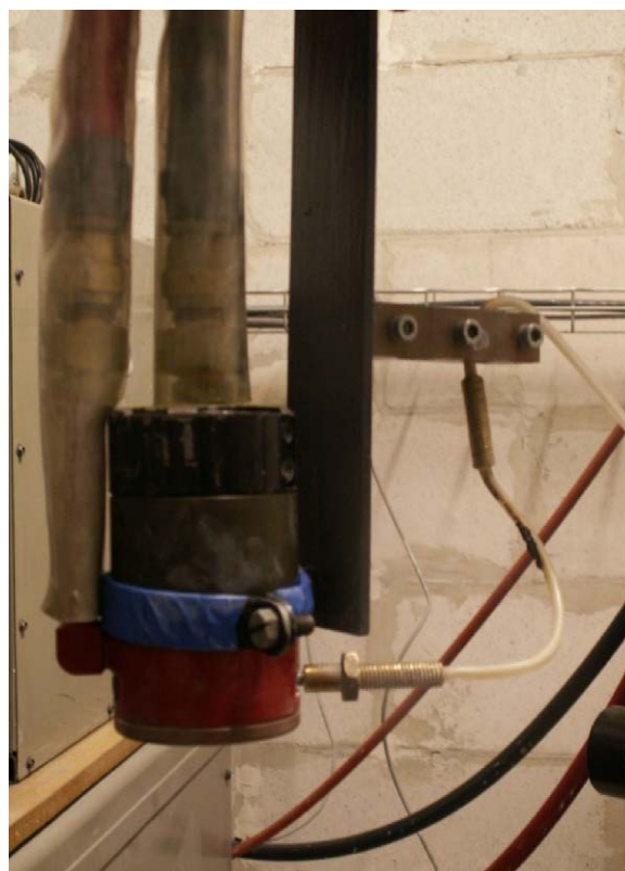
Fig. 4. Set up of internal injection mode with the use of continuous jet nozzle injector installed inside the plasma torch.
